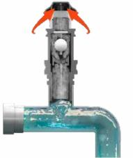
**Fluid draining phase** and air inlet into the system.
