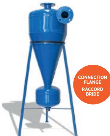
The **Hydrocyclone** separates sand and other heavier particles from the water. As a consequence of the centrifugal force, the solid particles move toward the cone wall in a downward spiral trajectory due to the force of gravity until they fall into the lower collecting tank where they are restored. The clean water exits the hydrocyclone through the tube at the top and the solid particles accumulated in the lower tank are periodically removed.
