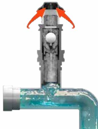
**Fluid draining phase** and air inlet into the system.
